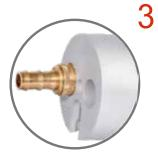
Place the coupling into the suitable coupling housing and make sure the accurate housing is installed on the tool. If not, please replace the housing with the other housing which you will find in the box.
